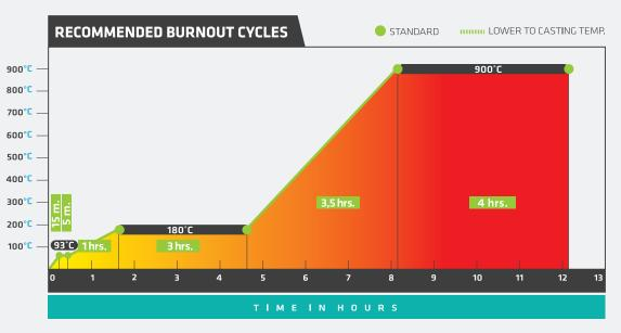
Reduce oven to the required casting temperature and hold for at least 1 hour, to stabilize the temperature throughout the flask before casting.
